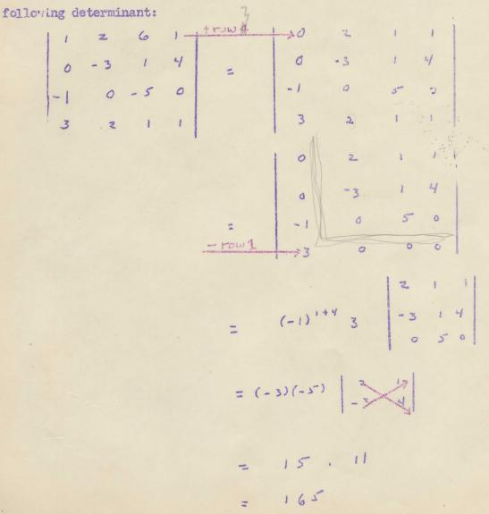
A systematic numerical method for evaluating a determinant is provided by the so-called reduction to triangular form: given the determinant
